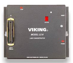
The **LC-8** Line Concentrator eliminates the monthly charges for dedicated phone lines to each elevator cab in an office, college, hotel, hospital, etc. A call initiated by any emergency phone is sent to the C.O. line. Subsequent calls activate call waiting tones to alert the emergency personnel that another phone has gone off-hook.
