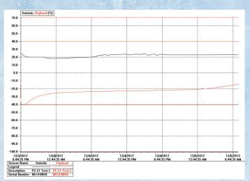
The red line indicates the payload area and the black line represents environmental temperature.
