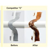
See nVent.com/FRICO for the terms of the Armour 10-year limited warranty. \* Salt-spray testing test method: ASTM B117 / DIN 50021; Cyclic corrosion test method: GM 9540P.
