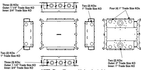
NOTE: Three (3) removable knockout plates per side allow for the EFB6S-2HUB 2" conduit adapter to be installed.
