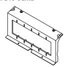
Mounting Bracket – Holds a standard 5 gang device plate Device plate dimensions: 10" x 4 1/2" [254mm x 116mm].
