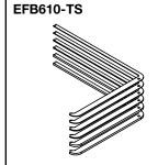
Tile Shim - Used for floor coverings greater than 3/16" [4.7mm]. The EFB610-TS allows the finished cover assembly to be flush with the finished floor. Includes one (1) 1/16" [1.6mm]. one (1) 1/8" [3.2mm] and one 1/4" [6.4mm] tile shims for 7/16" [11.1mm] of upward adjustment.
