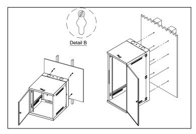
**Step 3**: Place the Wall Mount Cabinet onto the pre-drilled screws, then tighten all screws. Screws and screw slots should look like Detail B when fully tighten.
