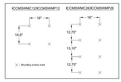
**Step 1**: Use a level to mark locations for mounting screws as shown above. Templates and screws are not provided.
