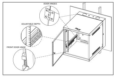
NOTE: To adjust the depth of the rail, lightly untighten the screw, adjust to the desired depth and then tighten the screw.
