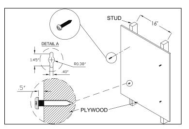
**Step 2**: Drill screws into marked locations without fully tightening them. Leave at least a .5" gap between screws and wall.
