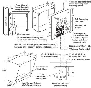
\*\* Note: Peel off paper liner and adhere gasket to the back of the faceplate, centering it over the mounting holes.
