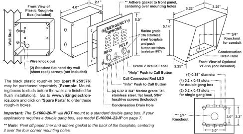
\*\*\* Caution: When warm air comes in contact with cold surfaces, such as outside walls and conduits, it causes condensation. To prevent condensation from accumulating inside the E-1600-20-IP always bring conduit into the bottom of the unit. If this is not possible, drill a 1/4" diameter hole in the bottom of the black plastic box.
