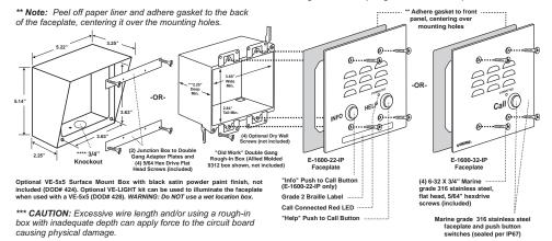
\*\*\*\*\* Caution: When warm air comes in contact with cold surfaces, such as outside walls and conduits, it causes condensation. To prevent condensation from accumulating inside the E-1600-92-IP or E-1600-32-IP always bring conduit into the bottom of the unit. If this is not possible, drill a 1/4" diameter hole in the bottom of the black plastic box.
