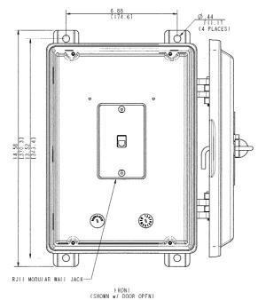
Note: Dimensions in Brackets are in Millimeters.
