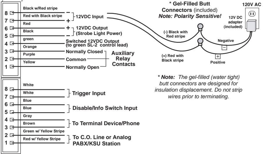
**\* Note:** The gel-filled (water tight) butt connectors are designed for insulation displacement. Do not strip wires prior to terminating.
