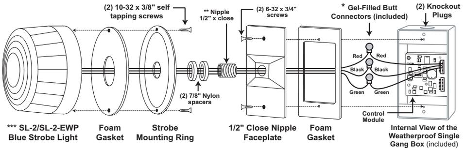
\* **Note:** The gel-filled (water tight) butt connectors are designed for insulation displacement. Do not strip wires prior to terminating.
