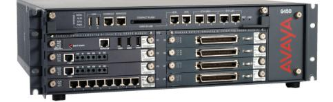
**Modular DSP Resources** are available as daughterboards for Main Board Module. These daughterboards can be implemented in increments. The maximum capacity is 320 channels. Codecs supported include G.711, G.729, and G.726.
