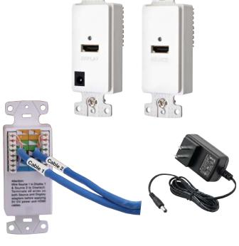
**Step 5:** Attach the 5V DC connector on the transformer to the DC input connector on the Display adapter.
