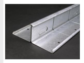
.040" [1.0mm] galvanized steel. Each base section has mounting holes, two 9/32" [7.1mm] diameter, located every 4" [102mm] and pass through KOs located every 8" [203mm] along the entire length. Packed four 10' [3.05m] sections of base per carton. Two DS4001 Couplings included with each 10' section.
