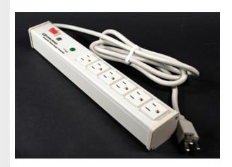
Perma Power computer grade surge protection. Six outlets, lighted switch, durable putty white aluminum housing, 15A. 15' [4.6m] 14/3 SJT putty white cord with NEMA5-15 plug. Length 16" [407mm]. Snap-on, slide-off mounting.
