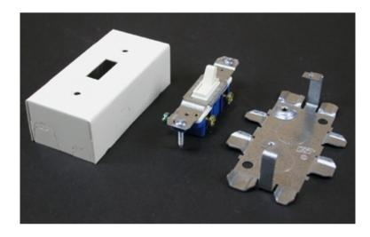
Single pole switch included. Accepts standard single-gang switches including three-way. Cover has twistouts for 500 or 700 Series Raceway on each end and sides. Twistouts on ends of box permit running raceway close to interior trim. Base has 1/2" trade size KOs. NOTE: Certified to Canadian Safety Standards for sale in Canada. When ordering these products, change the "V" color prefix to "vc" or the "WH" color suffix to "WHC" to denote the Canadian versions.
