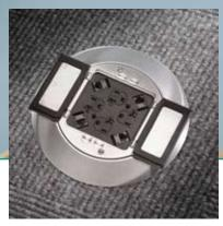
**4X4 Applications** Provides maximum power capacity for flush, multi-service applications. This sub-plate features a pre-wired four outlet 20A, 125V receptacle and four openings for snap-in flush mount Hubbell modular jacks and audio/ video snap-in connectors.
