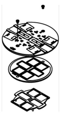
Nonmetallic slide holder assembly. Available in black (BK), gray (GY), ivory (VY), nonmetallic brass (BS), and nonmetallic aluminum (AA). Assembled with scrub water gasket. For use on tile or carpet floors.
