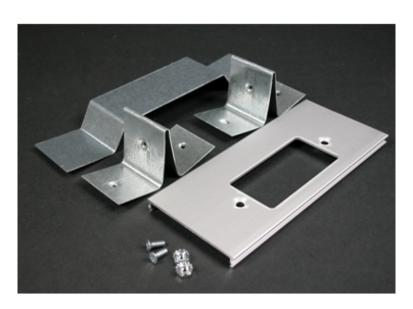
Installs rectangular devices including surge receptacles, GFCI, and other rectangular faced single-gang wiring devices in divided aluminum raceway. 6" [152mm] offset divider included. Can also be used with 106 communication frames.
