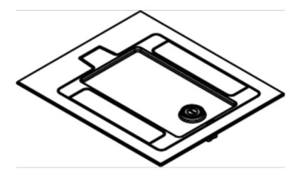
Cast aluminum cover assembly available in brushed aluminum (AL), painted black (BK), and gray (GY). Provided with carpet cut-out area. Maximum load capacity 1,500 lbs. UL Listed to U.S. and Canadian safety standards to meet UL requirements under UL514A for scrub water exclusion. NOTE: Not for use on bare concrete floor applications.
