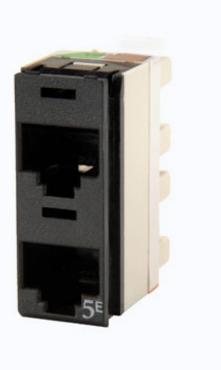
Clarity 5E dual panel jacks rear load into Ortronics maximum density 48-port 1 rack unit panel and exceed Category 5e component specifications. Rear load positive latch design, secures mounting of the jack into the panel. Universal T568A/B wiring label and tapered wiring towers simplify termination.
