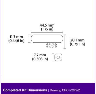
Note: To use fan-out kits with UniCam® Connectors, the installer must leave 4 mm of 250 µm coating.
