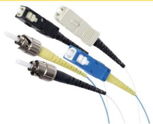
Hubbell's **2QUICK**® SC and ST-style connectors install in minutes. The **2QUICK**® connectors crimp easily on to 900 micron buffered fiber with a HPW hand tool. The fiber is then cleaved and the ferrule tip polished to produce a premium quality fiber connection. The **2QUICK**® Connector system eliminates the need for adhesives and expensive curing ovens and provides a reliable fiber optic connection. No epoxy or adhesives required.
