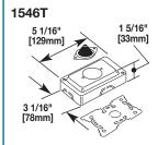
**Telephone Outlet Box** – Furnished with 1/2" [12.7mm] rubber stem. Accepts modular connecting blocks within the fitting. Cover has 1500 and 2600 twistouts on both ends and both sides. Two 1500WC wire clips included. Not UL Listed.
