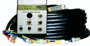
Specifications: (Typical @ 50 C) Length of cable: 25 meter/82 feet (cannot be shortened) Component video: Gain:  $\pm \frac{1}{2}$ dB Flatness:  $\pm 1/4$ dB 50Hz - 30MHz Skew: <1nsec S-Video and composite: Gain:  $\pm \frac{1}{2}$ dB Flatness:  $\pm 1/4$ dB 50Hz - 6MHz Isolation all cables >60dB
