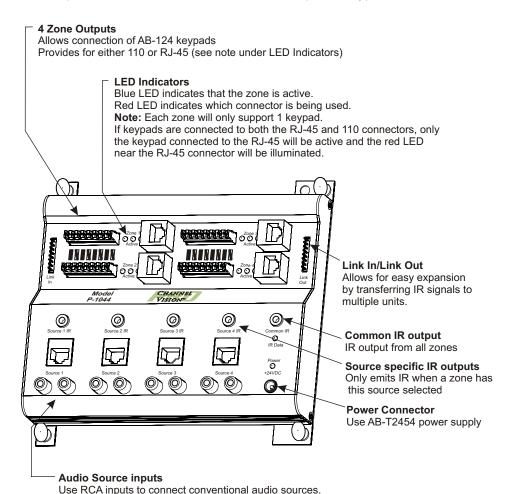
Use RJ-45 inputs to connect input modules such as AB-202, AB-301, and AB-311.
