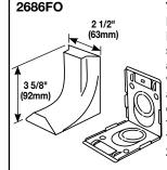
**Transition Feed Fitting –** Eliminates offsetting of 2400 Series Raceway in connecting with surface panel boxes. Has 3/4" and 1" concentric trade size KOs with 1" trade size KO elongated so adjustment from surface to center of bushing is 1" (25mm) minimum to 1 5/8" (41mm) maximum. Has twistouts for transition to 1500 and 2600 Series Pancake Raceways.
