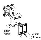
Divided Device Box - Divided two-gang, labor saving, over-theraceway box for use with 2400D Series Raceway. Provides the ability to have both power and low voltage at a single point-of- use. Accepts 5507 Series Faceplates, Ortronics® TracJack & Series II Modules (requires S2-EPL Plate), Pass & Seymour Activate Series Inserts (requires CM-EPLA Plate) and Wiremold CM2 Series Open System Communication Modules (requires CM-EPLA Plate).
