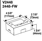
Device Box - One-gang device box. Cover has one twistout for 2400 Series Raceway on two sides and one twistout for 500 and 700 Series Raceway on the top and bottom. Base includes knockout to enable extension from existing single-gang flush wall box and 1/2" trade size KOs. Accepts industry standard faceplates for electrical and communication devices.
