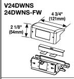
Device Plate - Accepts one Ortronics® Series II module.
