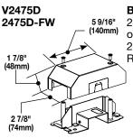
**Bridge Fitting** – For allowing 2400D Series Raceway to bridge over existing installations of 2400, 2400D, 500, and 700 Series Raceways.
