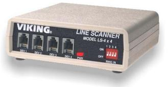
When a device, such as a modem, attached to a device port needs access to a telephone line, the **LS-4x4** will instantly scan for an open line starting from the last line to the first line. When the **LS-4x4** detects an open line, that line is routed to the device port, while incoming calls may also be routed to a corresponding device port. If no lines are available, a fast busy tone will be returned.
