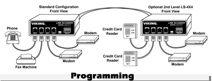
Incoming calls on each line can be routed to their corresponding device port by turning the appropriate dip switch on. *Note:* It is recommended that incoming calls be connected to the lower device ports.
