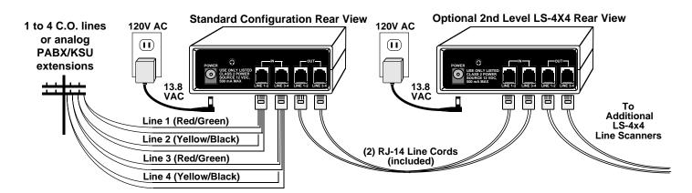
Note: Radio Shack part # 279-4011 combines two RJ-11's (one line) into one RJ-14 (two lines).
