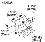
Single Receptacle Box - Accommodates commercially available straight blade and locking single receptacles with face diameters of 1.38-1.40" [34.5-35mm]. Base has 1/2" [12.7mm] and 3/4" [19mm] trade size concentric KOs. Cover has 1500 and 2600 twistouts on all four sides. Two 1500WC wire clips included.
