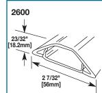
Base and Cover - Cover: .050" [1.25mm] galvanized steel. Base: .040" [1mm] galvanized steel. Packed (5) 10 ft. [3.050m] lengths per carton. Base has 9/32" [7.1mm] dia. mounting holes on centers of approximately 8" [203mm].
