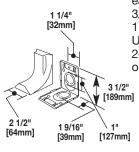
Adjustable Offset - Has twistouts for 2100 and 2600 on each end. Base has Connector 3/4" [19mm], 1" [25mm] and 1"[25mm] elongated knockouts. Use for 90° internal corners for 2600, transition from 2600 to 2100, or for connection to panel boxes.
