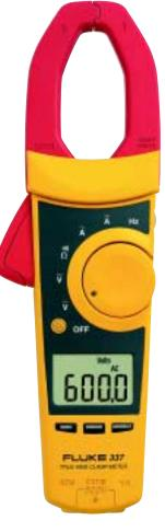
Fluke 337 The top-of-the-line True-rms clamp meter, large jaw measures ac/dc current and voltage, ohms, display hold, motor start-up current (in-rush), frequency, MIN/MAX capability and a large backlit display
