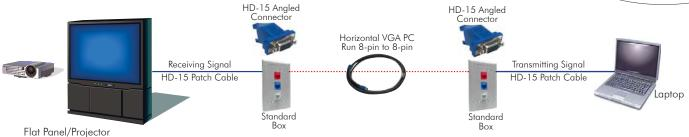
Application 2: Straight can be used with delivery exiting straight out the back (no constraints).
