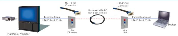
Application 4: 15 female to 8-pin horizontal run can be installed directly into the 1U VGA Module
