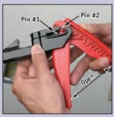
Angle handle so that pin # 2 will slide out first. Then slide out pin # 1.
