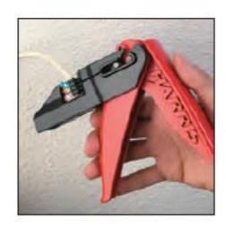
Ensure jack is completely and securely inserted in jack holder bed with IDC slots facing the blades.
