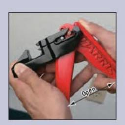
Open tool handle and move lever to pin #1 'down" position.
