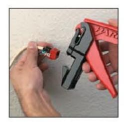
Insert jack in JackRapid front first with IDC slots facing blades of JackRapid.
