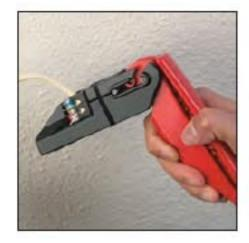
Pull trigger completely and remove excess wire prior to releasing trigger.
