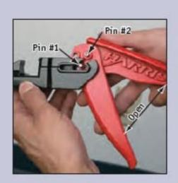
Angle handle, and insert pin one into blade head first. Be sure to keep tool handle in open position.
