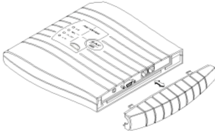
Figure 2-2 General View of the EAR 5000 after Removing the Cover
