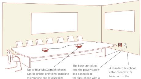
the first phone with a standard RJ-45 cable. telephone jack.
