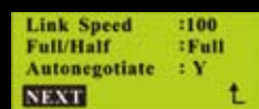
NETmapper connects to network at speed 100Mbps/Full duplex, and auto negotiation mode
