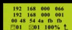
NETmapper's IP address (get from DHCP) Router IP address (Gateway) Router's Mac Address Counter for sending packages/Counter for receiving packages / the rate of package received
