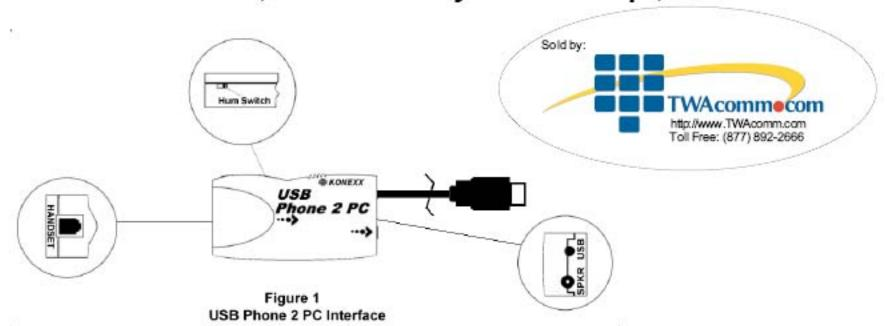
The USB Phone 2 PC interface has a small-unlabeled slide switch located on the side of the unit. This switch is called the "Hum Switch" (ref. Figure 1). The "Hum Switch" is normally not used. In some installations users may experience a hum or buzz in the recordings or on their telephone's receiver when the interface is connected. If this hum or buzz is experienced, the "Hum Switch" should be switched to the opposite side.
