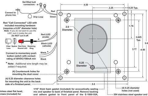
centering over speaker and microphone holes (as shown).
