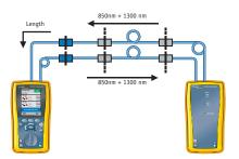
Unlike competitive fiber adapters which measure length and *two* loss measurements per Autotest, DTX is the only fiber test solution that measures length and *four* loss measurements per Autotest – all in about 12 seconds. With DTX Fiber Modules, you can speed through fiber testing five times faster than the competition.
