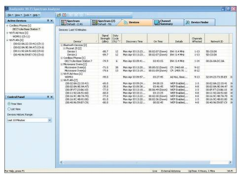
The Devices View shows detailed statistics for each device, including both currently active devices and historical devices.
