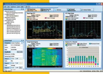
AnalyzeAir makes finding interference in 802.11 WLANs simpler by listing all active devices in the spectrum, both network devices and interfering devices. AnalyzeAir software wraps the tools RF experts use in an easy-to-use interface, putting the power of automated RF analysis into your hands.
