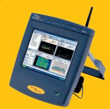
The wireless option extends the OptiView analyzer's capabilities; monitoring all 802.11a/b/g channels to capture and decode data packets, identify rejected association requests and pinpoint access-point conflicts.
