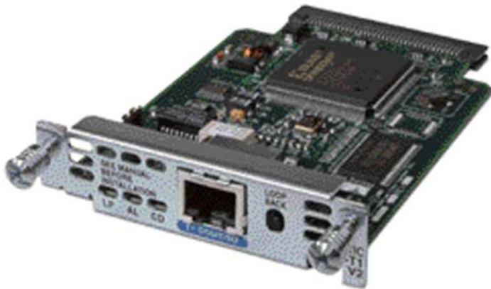
Figure 1. Cisco T1 DSU/CSU WAN Interface Card
