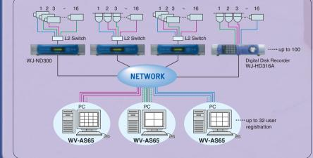
Remote control for multiple WJ-ND300 recorders via the network.
