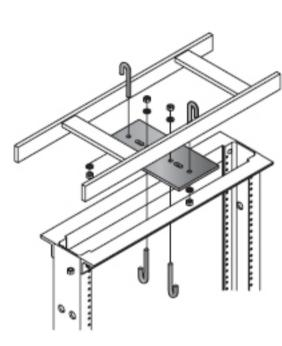
Note: 13730-X24 and 13731-X24 mounting plates add 1.25" to height of rack.
