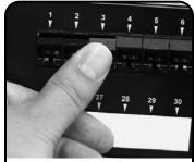
Install color-coded icons (as shown above) or hinged doors provided with modules into area above MAX modules to secure modules into panel. See MAX module instructions for additional
