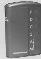
Personal Tactile Signaler AM-PXB for notification to the deaf/blind user through unique vibrating patterns and a tactile pad.
