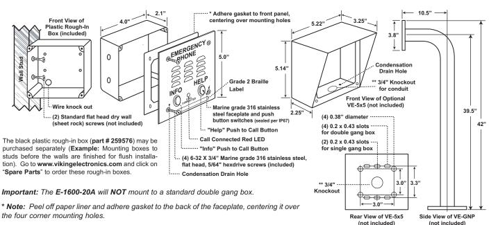
\*\* **Caution:** When warm air comes in contact with cold surfaces, such as outside walls and conduits, it causes condensation. To prevent condensation from accumulating inside the **E-1600-20A** always bring conduit into the bottom of the unit. If this is not possible, drill a 1/4" diameter hole in the bottom of the black plastic box.
