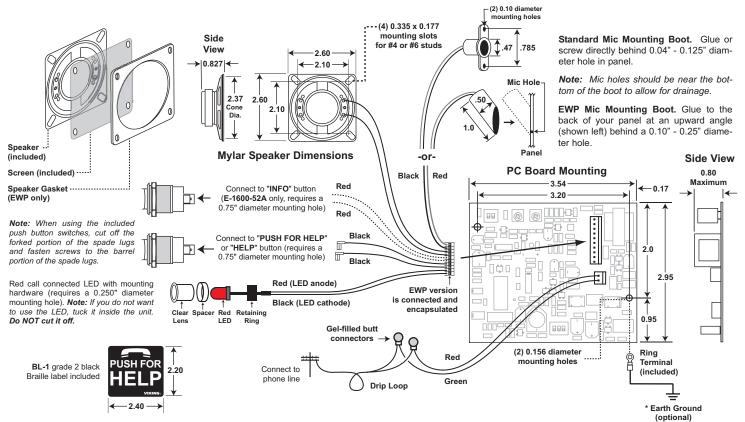
Important: If installing the EWP version outdoors, apply a non-corrosive silicone to back side of LED and push button switches after making all connections and testing. Completely encapsulate exposed switch connections (screw terminals/stripped wires) and bare wire connections.
