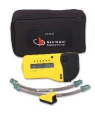
STM-8.....UTP (unshielded, twisted-pair) cable tester. Includes carrying case, remote "A", two universal modular plug cords, wiring guide, 9V alkaline battery, instructions, and warranty card
