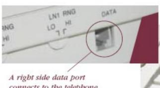
A right side data port connects to the telephone line for modem or fax machine use.
