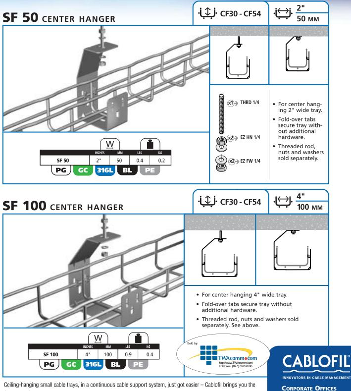
Ceiling-hanging small cable trays, in a continuous cable support system, just got easier – Cablofil brings you the SF 50 and SF 100. Attach bracket directly to deck or suspend from 1/4" threaded rod. Bracket secures tray with unique fold-over tabs. SF Brackets are available in a variety of finishes for extreme or exposed applications.
