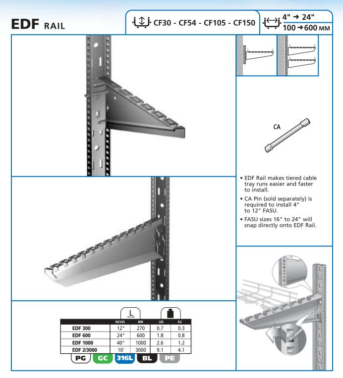
Speed installations of tiered cable tray runs with the new EDF rail from Cablofil. The FASU Bracket (4" to 12") requires a CA pin for attachment. The new FASU Bracket (16" to 24") snaps directly onto the EDF Rail for a secure and fast installation. A complete line of supports and braces makes EDF Rail the support of choice for any installation.
