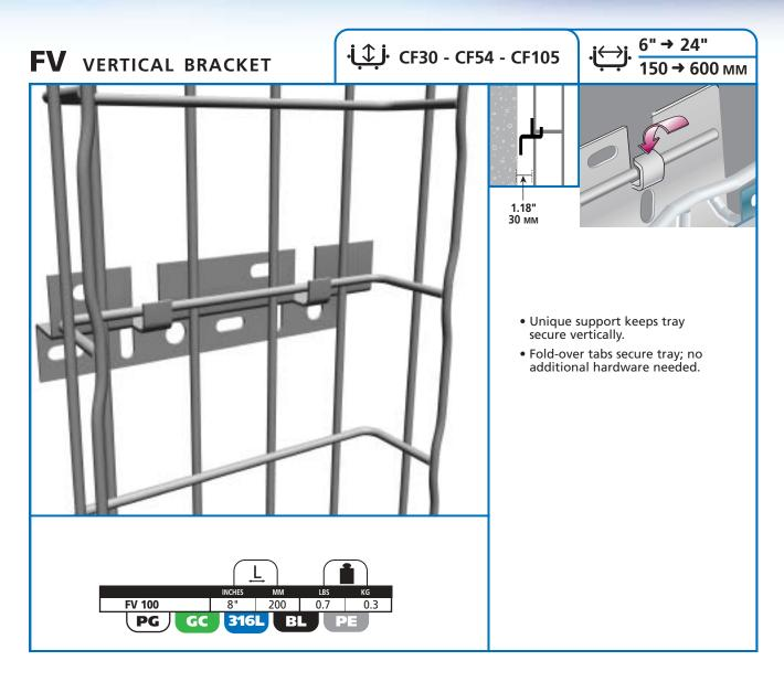
New from Cablofil, FV Vertical Bracket was exclusively designed to support vertical cable tray runs. Predrilled holes make attachment to walls or machinery easy. Unique fold-over tabs secure wire cable tray in place without additional hardware for faster install times.
