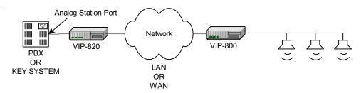
The VIP-820 Networked Trunk Port module can be used to create a multi-zone paging system from one Station Port of a PBX using existing corporate WAN. It provides up to 99 zones with two digit selection. When the VIP-820 sees an open loop disconnect signal from the PBX Station Port, the VIP-820 will release.
