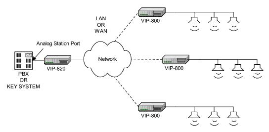
The VIP-820 Networked Trunk Port module makes it a snap to connect two or more PBX systems over the corporate WAN. It provides station to station PBX access, eliminating the need to use expensive trunk connections that are typically required by other competitive products. When the VIP-820 sees an open loop disconnect signal from the PBX Station Port, the VIP-820 will release.
