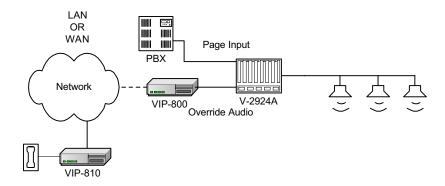
In this example, the VIP-810 and VIP-800 are connected to the data network as stand alone paging. This could be installed where network access is available, but not paging.
