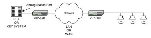
In this example, the VIP-810 and VIP-800 are connected to the data network as a stand alone paging system. This could be installed where network access is available, but telephone access is not.
