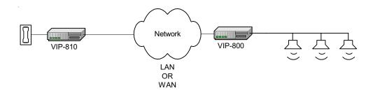
In these examples, two VIP-800's are connected to the data network to extend a paging zone to a remote location.
